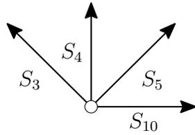
$$\begin{aligned}\uparrow: \quad S_5 \frac{\sqrt{2}}{2} + S_3 \frac{\sqrt{2}}{2} + S_4 &= 0 \\ \Rightarrow S_5 &= \frac{6\sqrt{2}}{5}G\end{aligned}$$
