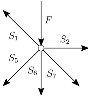
$$\begin{aligned}\nearrow: \quad S_2 \frac{\sqrt{2}}{2} - S_5 - F \frac{\sqrt{2}}{2} &= 0 \\ \Rightarrow S_2 &= \frac{12}{5}G + F\end{aligned}$$
